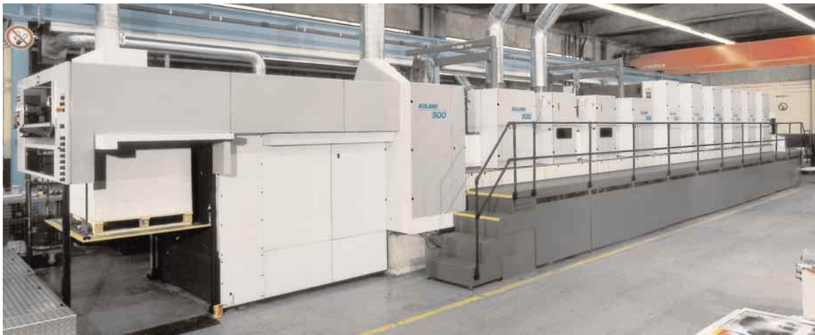
ROLAND 900: High technology for sheet-fed offset printing in broadsheet size.
