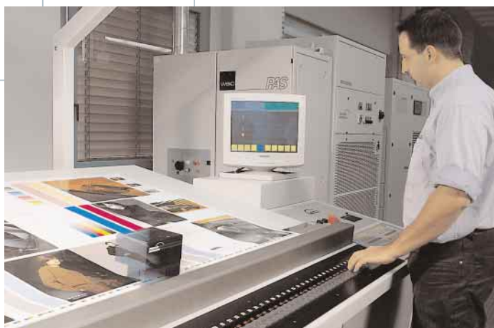
Selected ink feed from the RCI central control console quickly and without problems.
