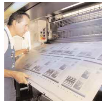
The automated PPL Plate Loading system allows the plates to be clamped easily in the perfecting unit.
