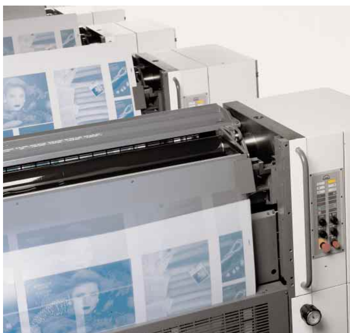
Automatic change of plates for considerably reduced makeready times.
